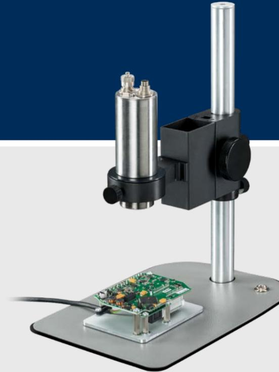
The microscope optics for the Xi 400 allows reliable temperature measurement on tiny objects from 240 µm. In combination with a suitable stand, this enables professional measurement of printed circuit boards and components in the electronics industry.
