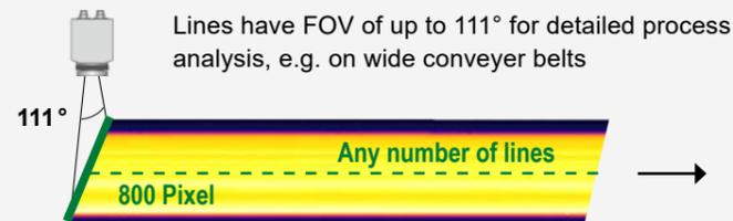
Up to 32 Hz data recording\* of unlimited lines which in turn produce a thermal image of any given resolution.
