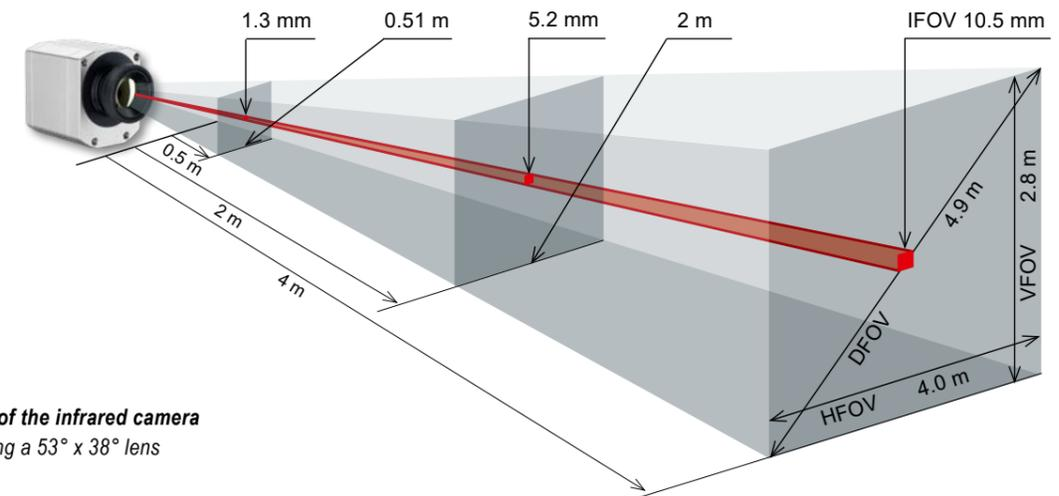
Measuring field of the infrared camera
