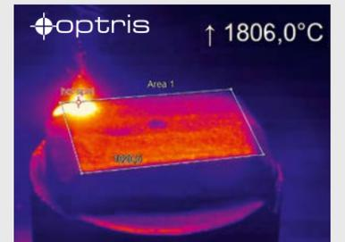
Measurement during laser welding process
