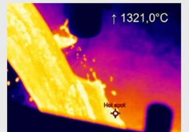
Measurement of a pouring stream
