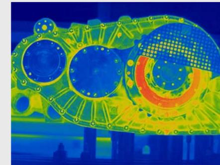
With a thermal resolution of 40 mK, the optris PI 450i is used for measuring the most subtle temperature differences, e.g. in the quality control of products or in preventive medicine.
