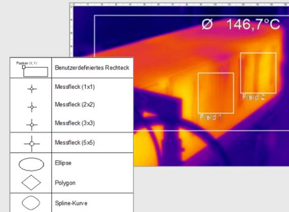
The size and shape of measurement area can be freely designed and moved. For an easy introduction, a large selection of pre-defined measurement area shapes is available.
